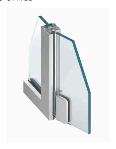
• The structural depth of profiles is 45 mm, which is identical to the depth of profiles of all the frames and studs of the MB-45 system. Both solutions are fully compatible, which allows to freely combine their profiles. The MB-45 OFFICE is based on a profiles, which after tightening the appropriate adaptive profiles can function as a window or door frame, a transom or a stud. The system is compatible with hinges, locks and automatic door closers manufactured by Aluprof, Gezeand WSS.
