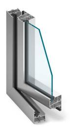
• The structural depth of the window sections is 45 mm (frame), 54 mm (sash) and the door: 45 mm and 45 mm, respectively. Such assumed depths of the sash and frame give the effect of one surface on the external side after closing - in the case of the window, and the effect of adherence to the surface of the sash and frame in the case of the door. The shape of the profile allows slender and resistant window and door constructions to be obtained.
